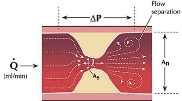
$$\Delta \mathbf{P} = \underbrace{\mathbf{f}_1(\mathbf{I}_{As^2}, \mathbf{Q}, \dot{\mathbf{Q}})}_{\text{Viscous}} + \underbrace{\mathbf{f}_2(\mathbf{I}_{As^2}, \mathbf{I}_{An^2}, \dot{\mathbf{Q}}^2)}_{\text{Separation}}$$
